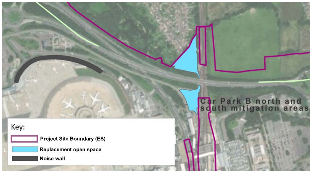
Figure 59: Car Park B: Areas to be Converted from Carparking to Landscaped Areas
